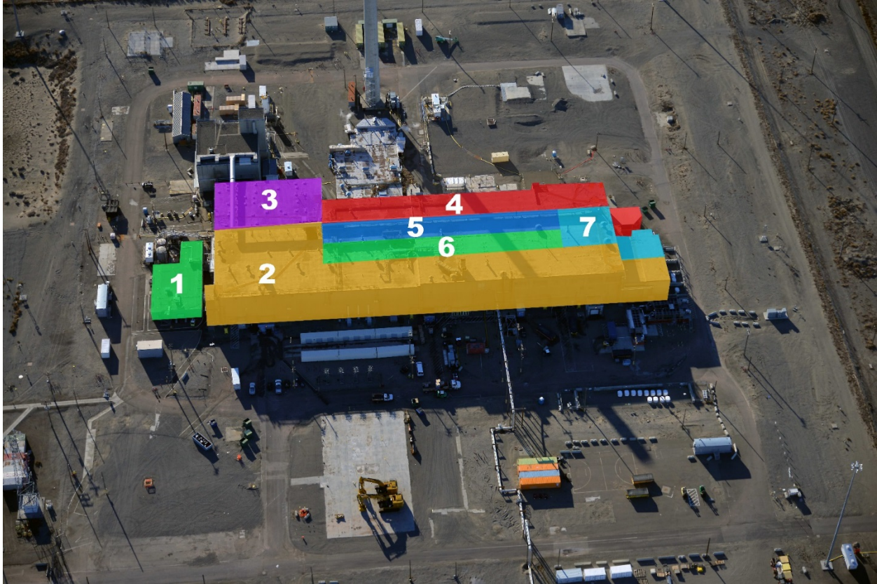
Figure 2: This illustration shows the seven zones and sequence for demolition of 234-5Z.
